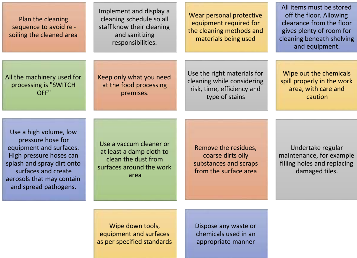
Fig. 2.2.4 Standard Practices for Cleaning the work area and equipment
