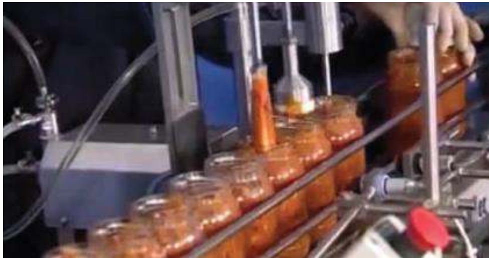
Fig. 4.4.4. Bottle filling machines used for filling of juices squashes into bottles
